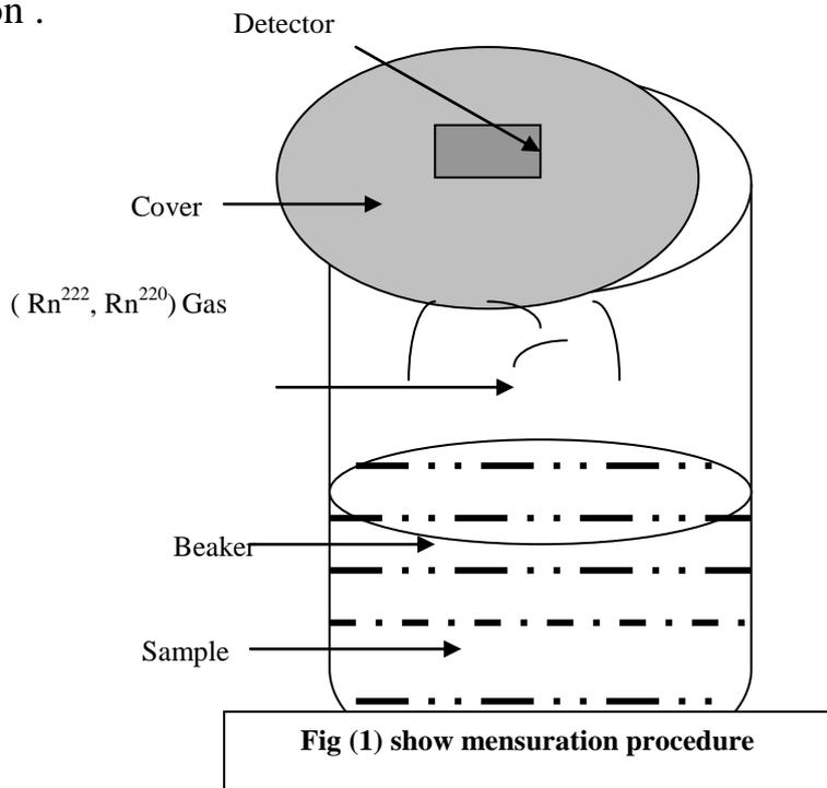
between radon and other isotopes. After that, the cups were changed by cups containing the detector on the top and again enclosed onto the samples. After 45 day periods, the detectors collected and non-destroyed ones were analyzed.
